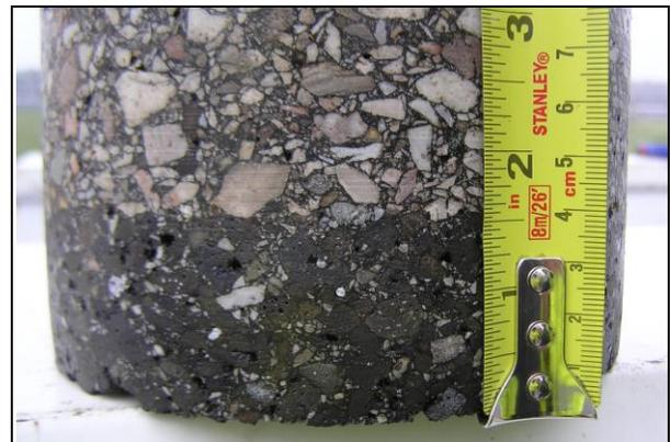
*Core showing the 9.5 mm steel slag surface course (darker colored lift).*
